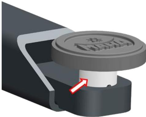
The thread on the support plate is used for height adjustment so that the vehicle rests evenly on all four support plates during lifting. This thread must be smooth-running. Dirty threads should be cleaned and lightly greased. The retaining ring on the underside must be present and correctly fitted.
