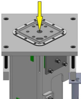
2 Loosen the screw plugs of both lifting units by max. one turn.
