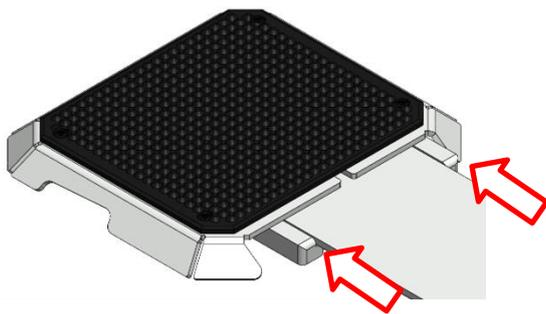
The sliding surfaces of the flat head pull-outs must be relubricated every six months at the latest.
