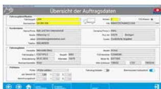
The input screen for vehicle and owner data can directly access the SQL database.
