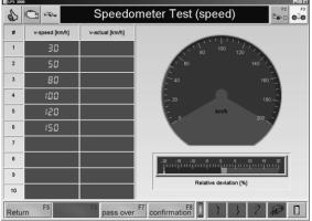
Use the <F5 RETURN> to jump back to the previous target speed. Use the <F7 PASS OVER> key to jump to the next target speed.
