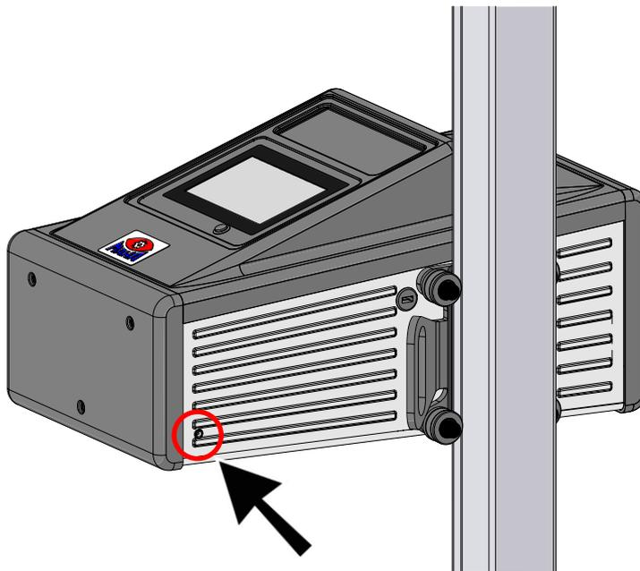
A normal charging process takes approx. 11 hours. The full battery capacity is reached when the charging current has dropped to 0.00 A.
