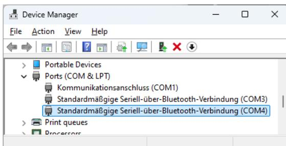
Open the Device Manager and check the COM interface for the Bluetooth connection under 'Ports (COM & LPT)'.
