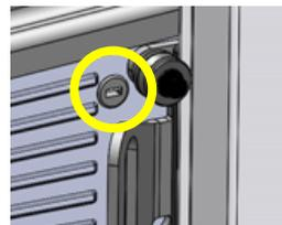
Connect the USB stick to the USB port at the outside of the casing.
