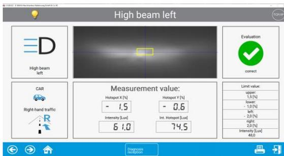
The selected measurement data is displayed in detail.
