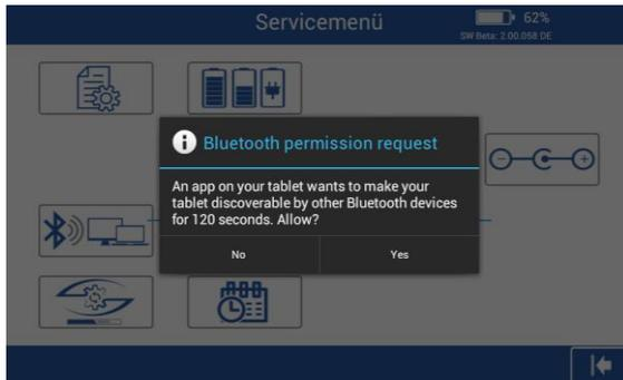
Confirm the request with 'Yes'. The headlight tester is now discoverable by other Bluetooth devices for 120 seconds.
