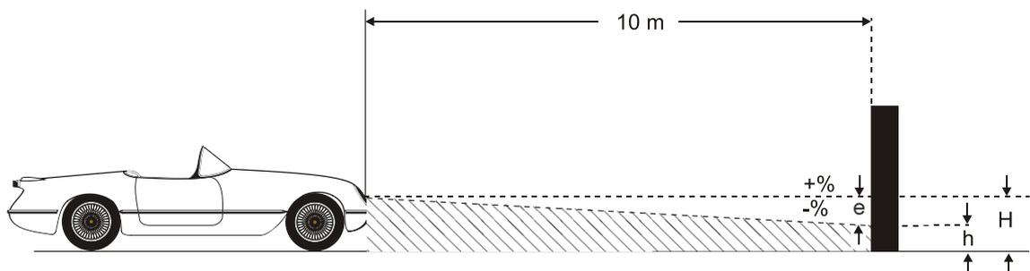
The inclination of the light-dark limit against the test surface is expressed as a percentage, using 10 m as a reference parameter:
