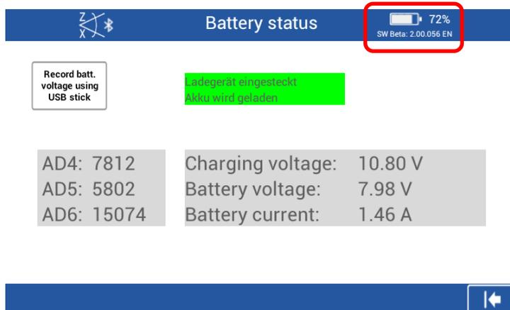
Record batt. voltage using USB stick
