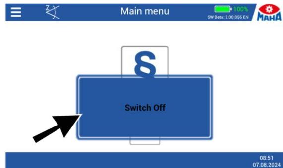
After pressing the button, confirm 'Switch off' on the touchscreen.
