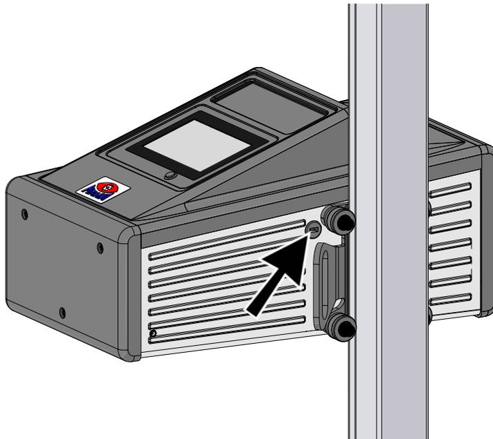
To record this data, a USB stick is required, which is plugged into the USB-A socket on the outside of the housing.
