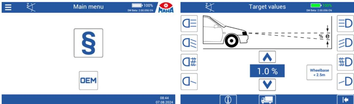
To start the measurement, press the desired light button.
