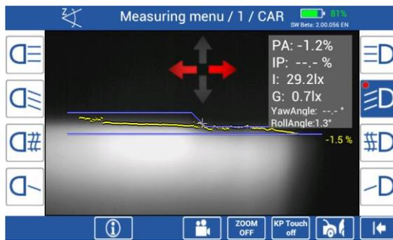
If the inflection point is incorrectly or not recognised (red arrows to the left and right), the inflection point can be set manually.
